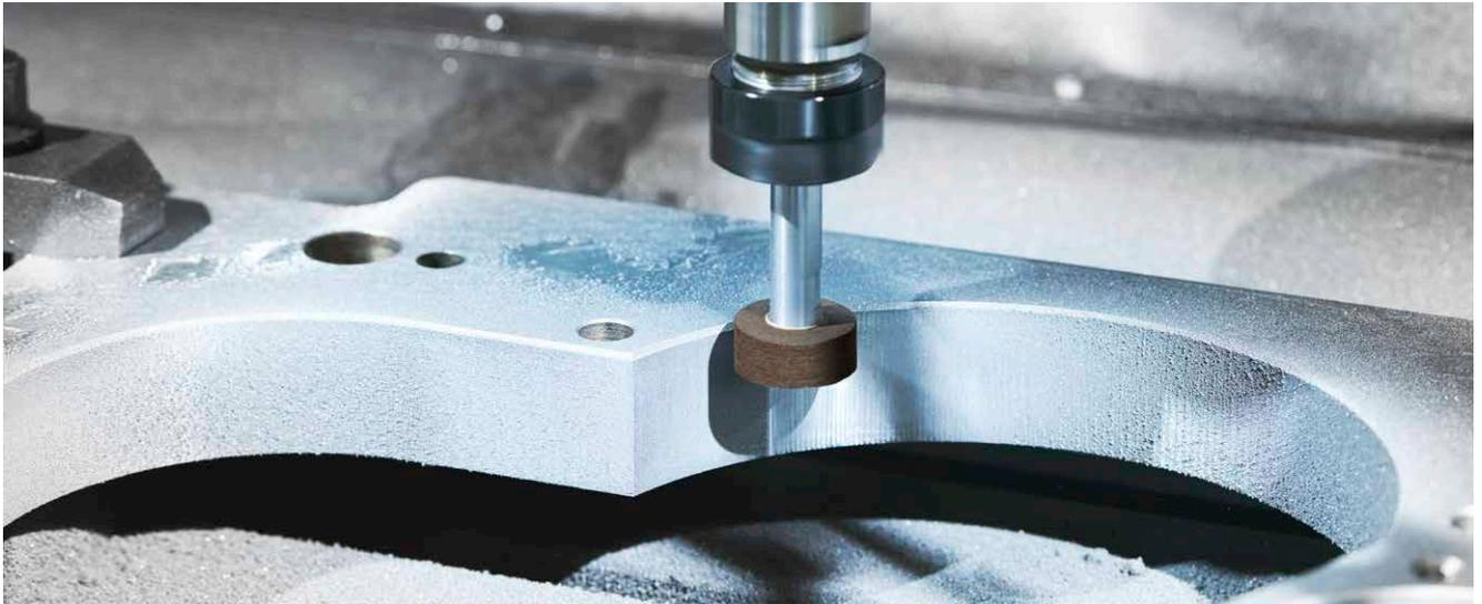
These polishing points are available in one grit combination only. The surface finish is similar to a finish with grit size 100. The hard rubber bond makes these points particularly suitable
