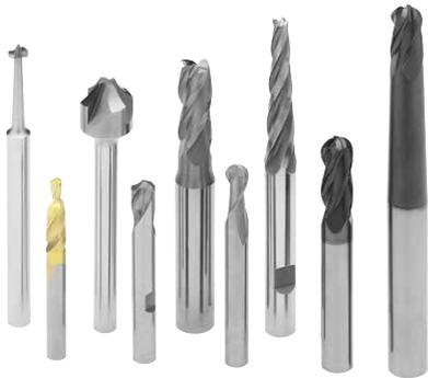
In addition to rotary burrs, we also produce tungsten carbide milling tools in special shapes and sizes for stationary applications. We supply these milling cutters with a maximum diameter of 20 mm and a maximum length of 250 mm; they differ from our extensive standard range in their shape, tool material and geometry (rake, clearance and helix angles).
