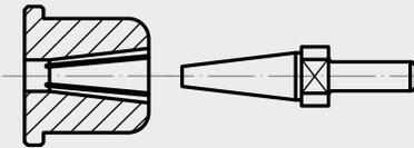
The mounting system for polishing wheels consists of a plastic sleeve (MCA) and a mounting arbor with 8 mm diameter shank (K25), which is solely applicable to shape SE1 in the dimensions 10010 B 25 and 10020 B 25. This system is not designed to be used for polishing wheels with larger diameters. The maximum cutting speed for this mounting system is 10 m/s. This results in a maximum spindle speed of 1900 rpm with a wheel diameter of 100 mm.
