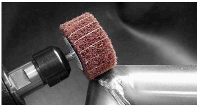
These LUKAS grinding tools feature a combination of abrasive fleece and abrasive cloth. During the production, the fleece and cloth flaps are fastened alternately and radially to the tool axis.
