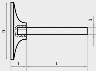
The GTH abrasive disc carriers with diameters of 18 and 30 mm have Inox hooks. Hooks with a diameter of 45 mm and greater are made of polyamide.
